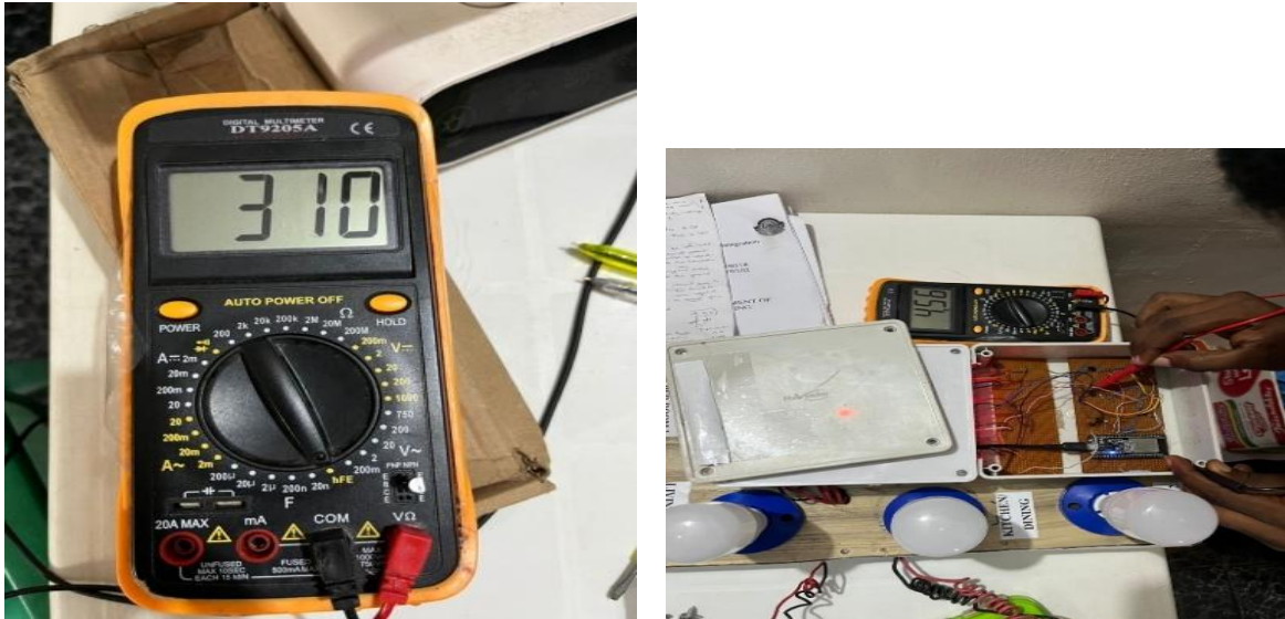
Figure 5: transistor measurement (a) the h_{fe} measurement and the (b) collector current measurement
